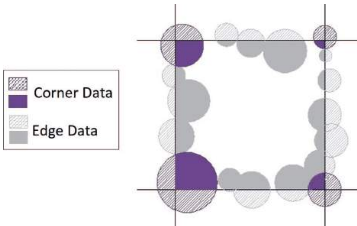
Figure 5. A schematic of a tile with the two types of boundary data. The solid-colored tree crown pieces inside the tile should be unified with the corresponding stripe-colored parts outside in a distributed computing environment.
