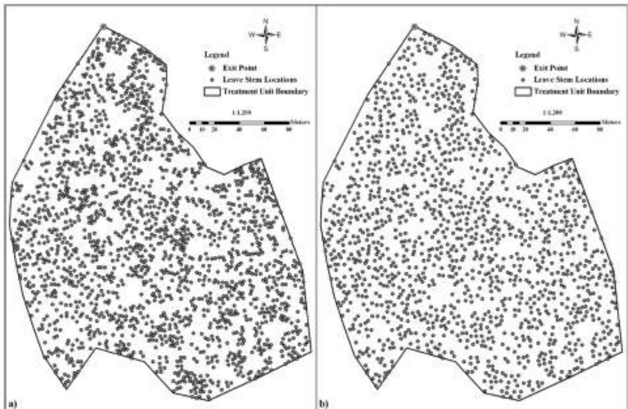
Figure 7. Leave-tree locations after manually selected cut trees were removed under the two thinning scenarios, with target densities of 400 (a) and 300 (b) trees/ha.
