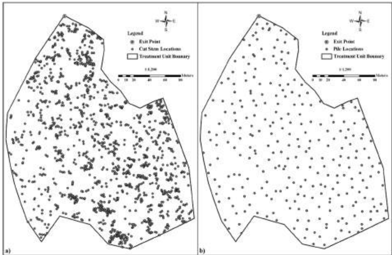
Figure 12. Cut-tree locations under thinning scenario II (a) and the corresponding log-pile locations identified by the log-bunching algorithm (b).
