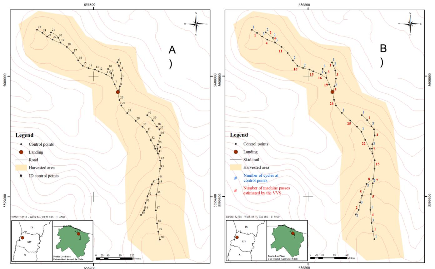
Fig. 4. Area used to test the application of the tool, with the location of the 54 control points (A), and the simulated log pile locations and number of machine passes per skid trail segment (B).
