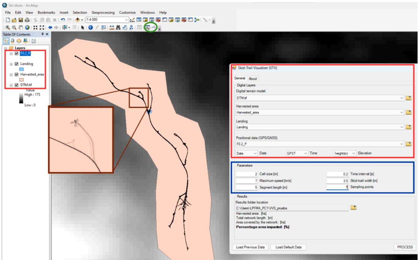
Fig. 5. Input data (digital layers and parameters) loaded into the graphic user interface of the computational tool.
