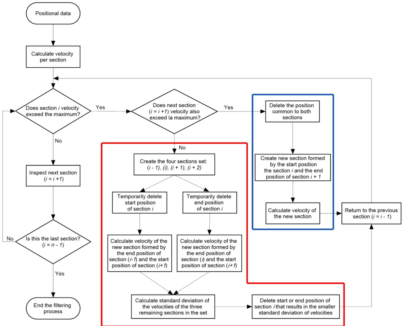
Fig. 1. Flow chart of the logical process used to filter outlier positions.
