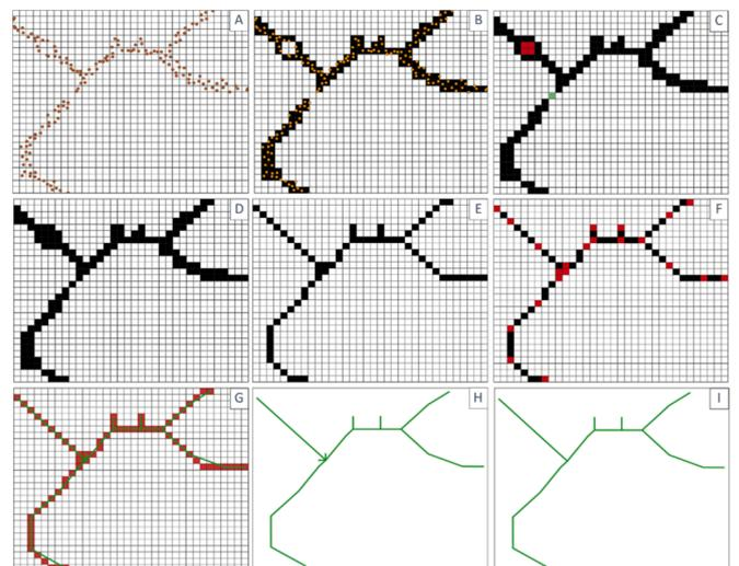
Fig. 3. Diagram of the skid trail generation process used by the computational tool.
